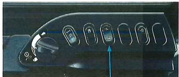
Attachment selector switch
