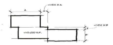
This diagram is an example of how separate Building Elements could maintain compliance with the square foot maximum called for, while being part of a larger structure. The block below and to the right of the uppermost block is attached to a wall the length of A and is offset by 15% of the length of A. The block to the right and slightly below the second block is attached to a wall the length of B and is offset by 15% of the length of wall B.
