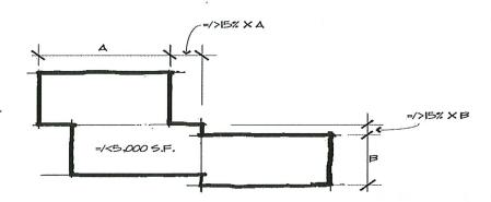
This diagram is an example of how separate Building Elements could maintain compliance with the square foot maximum called for, while being part of a larger structure. The block below and to the right of the uppermost block is attached to a wall the length of A and is offset by 15% of
