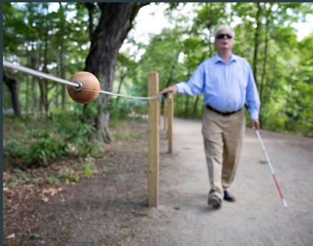
Above, a spherical block on a cable alerts a braille trail user in Watertown, MA that there is a bench opposite. (image credit Robin Lubbock/WBUR)
