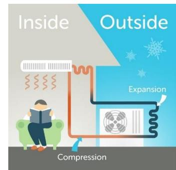
Figure 6-B.4: Illustration of how cold-climate heat pumps work. Source: Efficiency Vermont.
