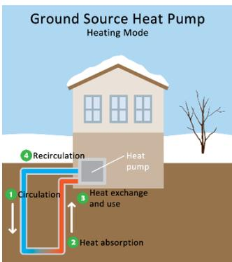
Figure 6-B.5: Illustration of how ground-source heat pumps work. Source: US EPA.
