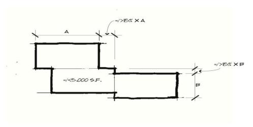
This diagram is an example of how separate Building Elements could maintain compliance with the square foot maximum called for, while being part of a larger structure. The block below and to the right of the uppermost block is attached to a wall the length of A and is offset by 15% of the length of A. The block to the right and slightly below the second block is attached to a wall the length of B and is offset by 15% of the length of wall B
