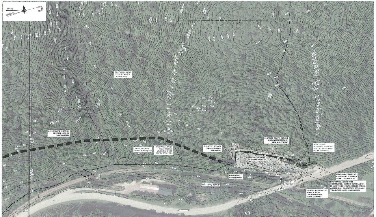
PURPOSE OF PLAN: THE PURPOSE OF THIS PLAN IS TO CLOSE THE EXISTING OUARRY OPERATION AND CONSTRUCT A CONTRACTOR YARD IN THE SAME LOCATION. THE GRADE OF THE SITE IS PROPOSED TO BE LOWERED AND A NEW ACCESS LOCATION IS PROPOSED ONTO VITIO3. THE PROPOSED LAYOUT IS INTENDED TO ALLOW ADEQUATE CIRCULATION FOR VEHICLES INCLUDING BUT NOT LIMITED TO TRACTOR TRAILERS (AASHTO WB-67).
